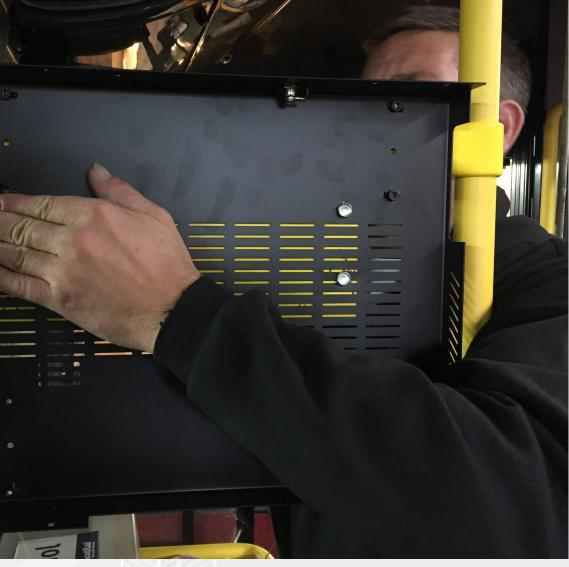
Once the mounting bracket for the AV Monitor has been secured to the yellow mounting plate on the pole, then the AV Screen can be secured to the bracket.
